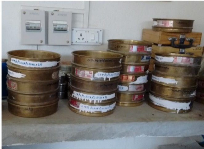
Fig 2. Various sieve for sieve analysis
