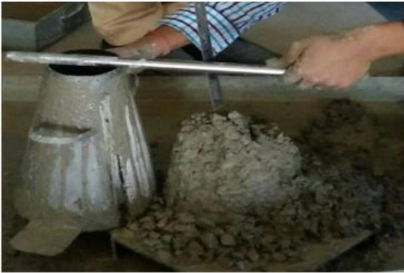
Fig.3. Workability test (Slump test)
