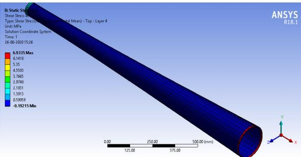
Figure 2: Shear stress for carbon epoxy for layer 4 top side
