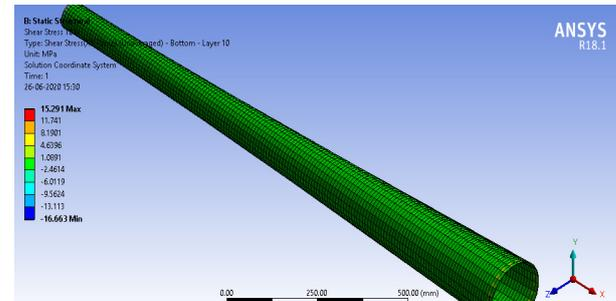
Figure 8: Shear stress for carbon epoxy for layer 10 bottom side
