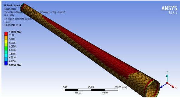
Figure 1: Shear stress for carbon epoxy for layer 1 top side
