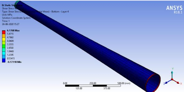
Figure 3: Shear stress for carbon epoxy for layer 4 bottom side
