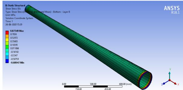
Figure 6: Shear stress for carbon epoxy for layer 8 bottom side
