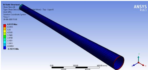
Figure 4: Shear stress for carbon epoxy for layer 6 top side
