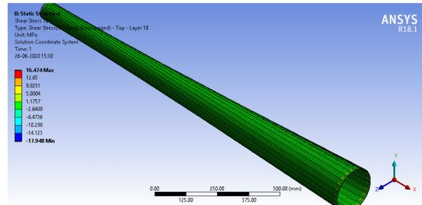
Figure 7: Shear stress for carbon epoxy for layer 10 top side
