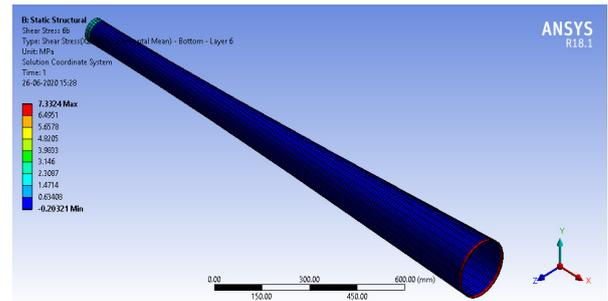
Figure 5: Shear stress for carbon epoxy for layer 6 bottom side
