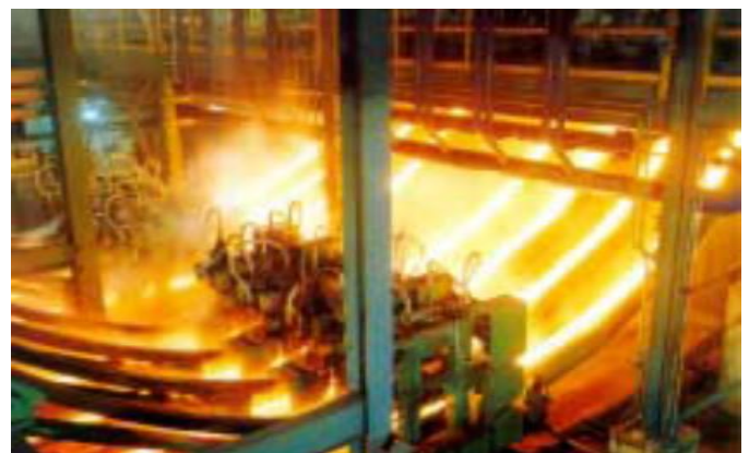
Figure-4: Hot strands passing through cooling chambers in a circular arc
