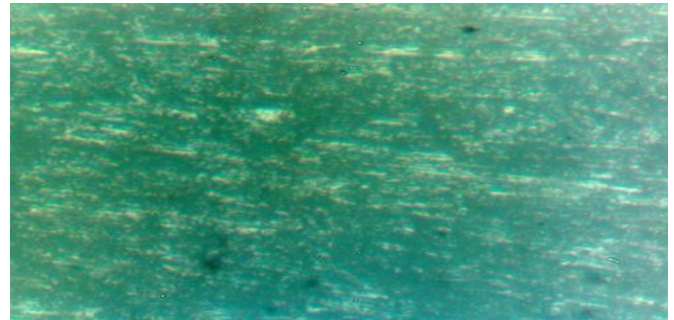
Fig. no – viii. Microstructure of AA 7075 with reinforcement of 0.25% nano SiC
