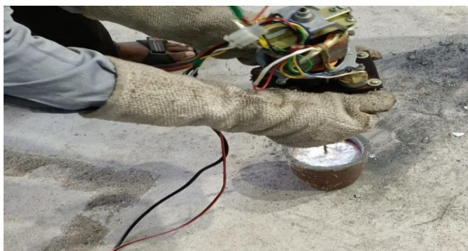
Fig no.- ii. After adding reinforcement stirring of liquid aluminium.
