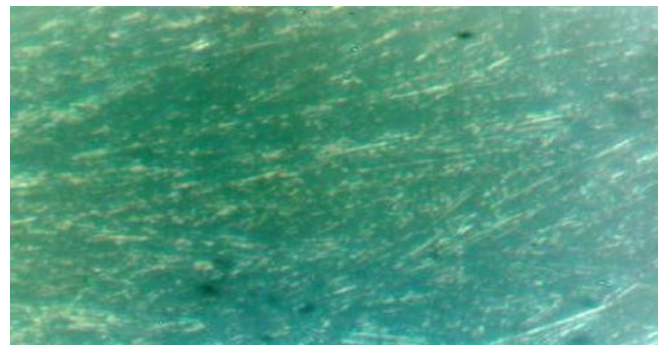
Fig. no. – x. Microstructure of AA 7075 with reinforcement of 0.75% nano SiC
