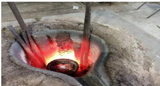
Fig. no.- i. Melting of al in-furnace
