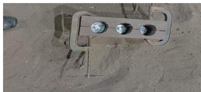
Fig no.- iii. Casting in permanent mould
