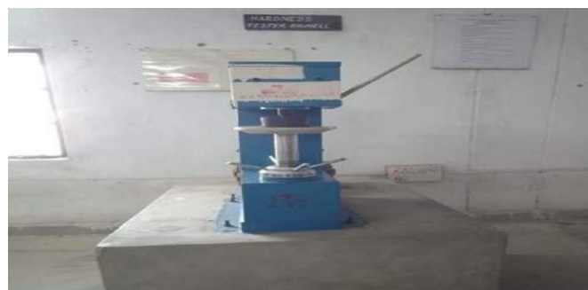
Fig no.- v. Brinell hardness testing machine
