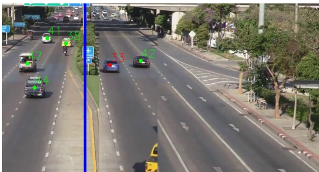
Figure 4. One of the violations stored in Firebase (red colored centroid indicates a violation and the blue line is the imaginary median automatically constructed by the program)
