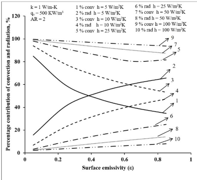
Figure 11: Relative contributions of convection and radiation to cavity heat dissipation for different surface emissivities in various regimes of convection
