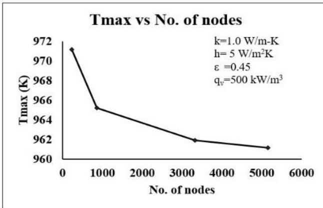
Figure 4: Variation of maximum temperature of the cavity with number of nodes
