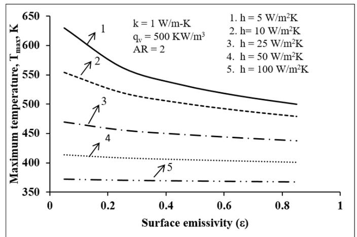
Figure 7: Variation in maximum temperature of cavity with emissivity in distinguished regimes of convection
