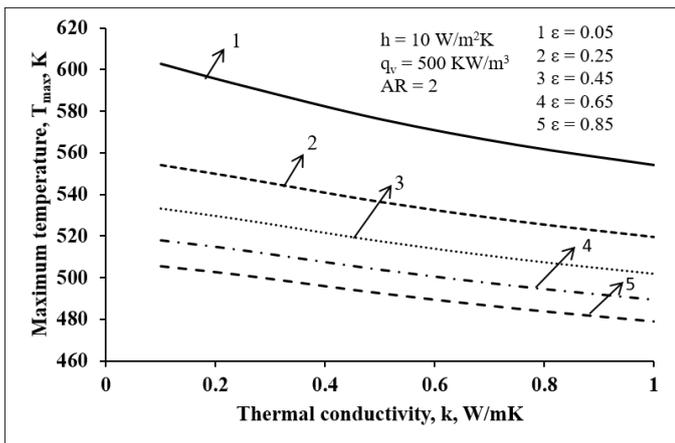
Figure 9: Variation in maximum temperature of cavity with thermal conductivity of cavity material
