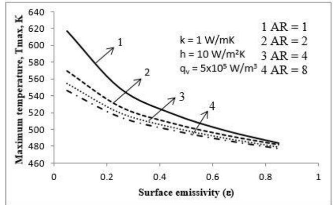
Figure 12: Maximum temperature variation with aspect ratio for different surface emissivities
