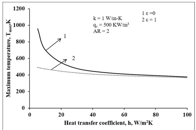
Figure 10: Role of radiation in distinct regimes of convection on maximum temperature of cavity
