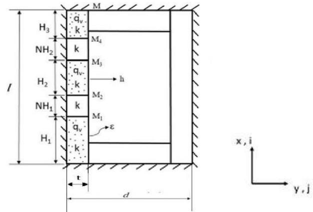
Figure 1: A rectangular closed cavity with multiple non-identical discrete heat sources along with its coordinate system
