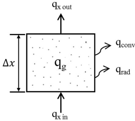
Figure 2: Energy interactions at the interior heat source elements of left wall of the cavity
