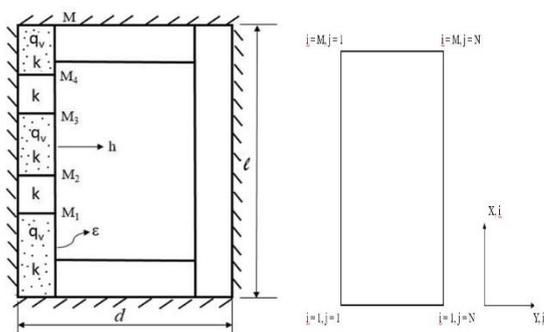
Figure 3: Computational domain of the problem geometry along with node representation
