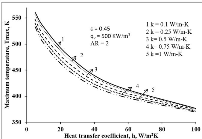
Figure 8: Variation in peak temperature of cavity with convection heat transfer coefficient for different materials of the cavity
